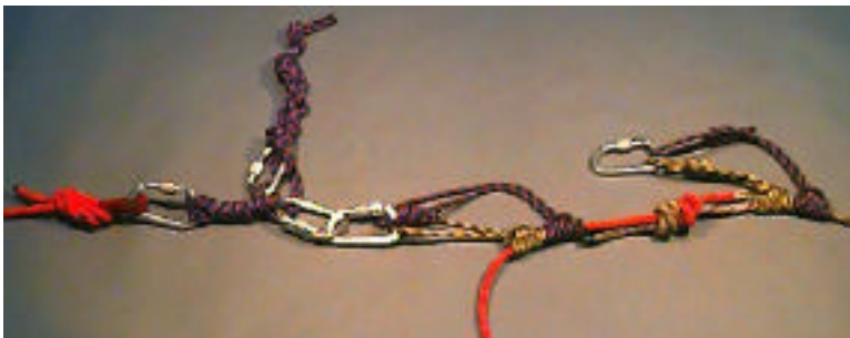
Figure 8 – Ready to pass a bend in the line.
