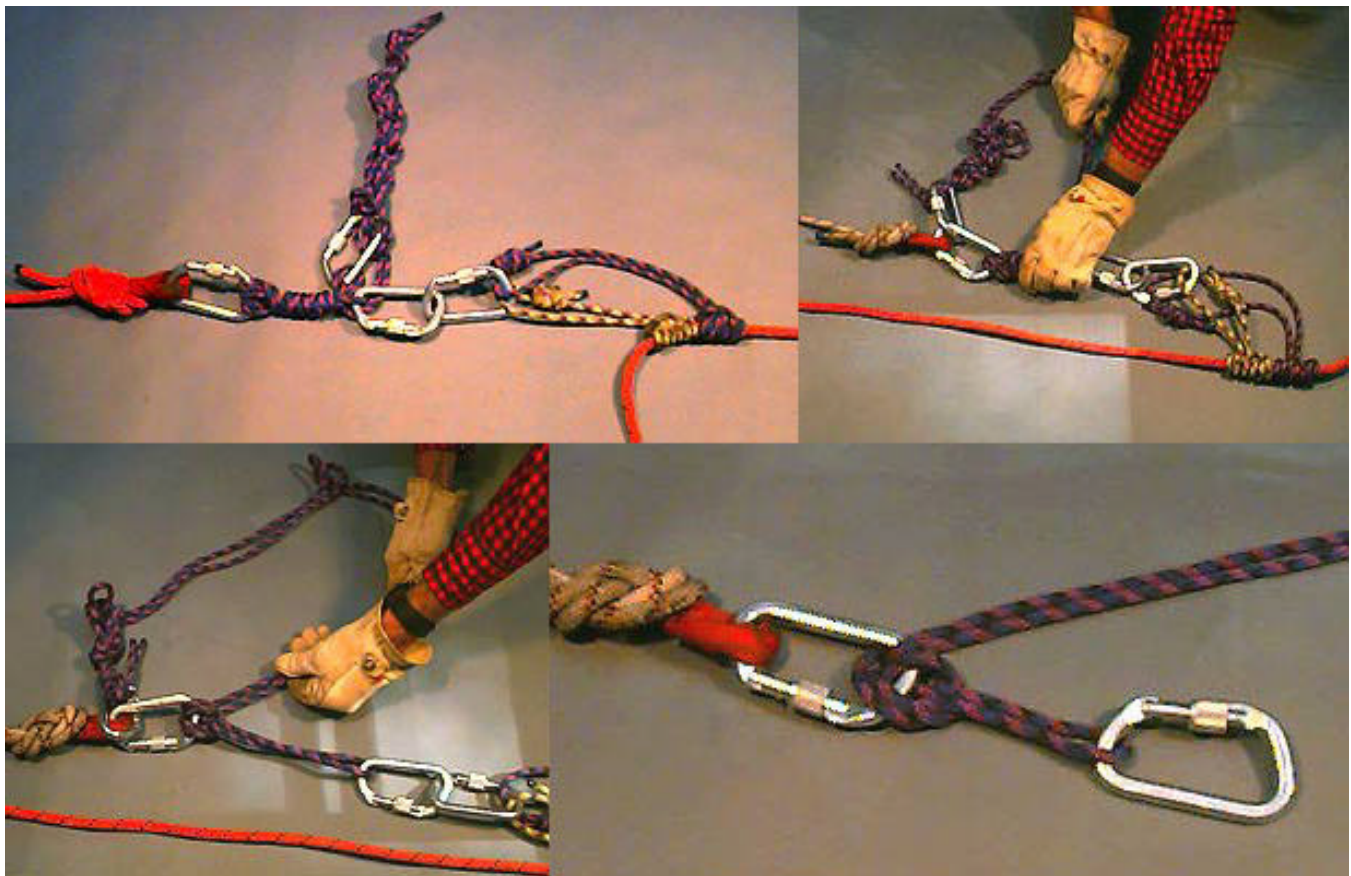
Figure 12 –Tandem Prusik belay attached to the belay line, load release hitch at the ready. (Top left) Starting to release tension with the load release hitch. (Top right) Load release hitch unwrapped, using the Münter or Italian hitch to release tension. (bottom left) The guts of the load release hitch, a Münter or Italian hitch. (Bottom right)
