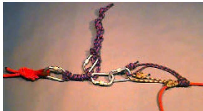
Figure 6 - Tandem Prusik belay attachment, before rigging to belay line and attached to the belay line.
