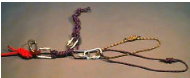
Figure 6 - Tandem Prusik belay attachment, before rigging to belay line and attached to the belay line.
