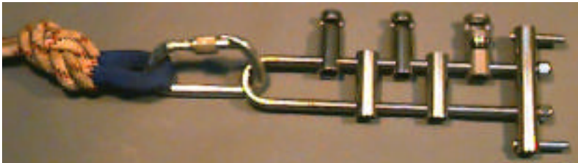
Figure 3 – Break bar rack, before rigging.
